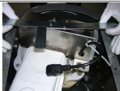
7 Lift up drive motor and bracket assembly
