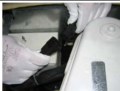
4 Unplug the drive motor connections...
