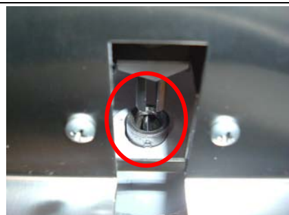
14 Pay attention to match drive motor shaft with bin vane shaft pin when place again the drive motor assy
