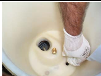
12 Clean/sanitize inside storage bin
