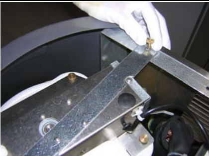
5 Unloose the top bracket holding screws
