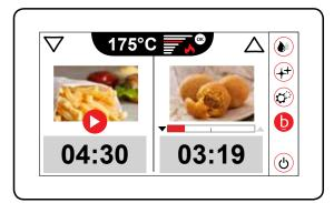
Operating menu screen showing cooking times for the selected recipe and current tank temperature.
