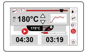
Option of adjusting standard settings and viewing tank temperature progression. Option of setting the melt cycle.
