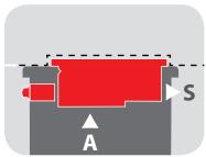
S = Exhausted air vent A = Suction / Cooling
