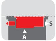
S = Exhausted air vent A = Suction / Cooling
