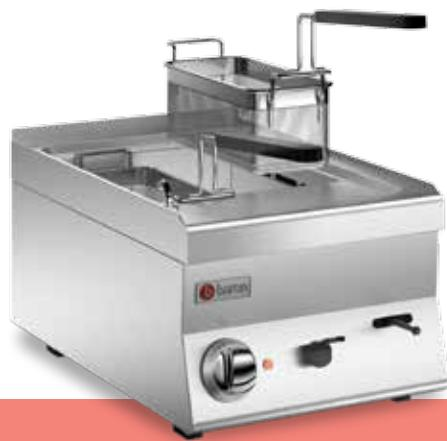
These appliances are equipped with high power to maintain the water at boiling point. The tray has a sufficiently wide surface to make sure that the foam formed by the dissolved starches drains away and stops it from leaking out. The appliance has a safety thermostat and an operation light.
