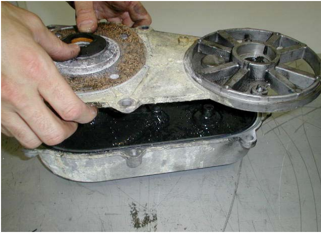
10. Remove the Gasket and ...
