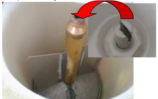
26. Reinstall bin cover holding the agitator motor paying attention that grooved are of the agitator motor 's bracket meets metal pin fitted at the upper part of the agitator bracket.
